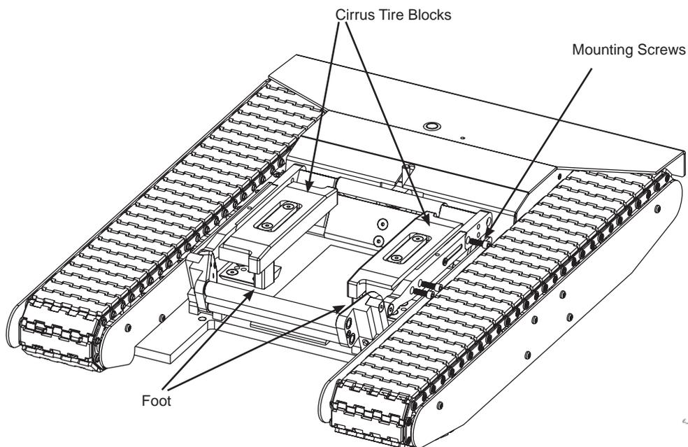
3. Loosen the 2 clamp screws on each spacer block to adjust for your tire width.
