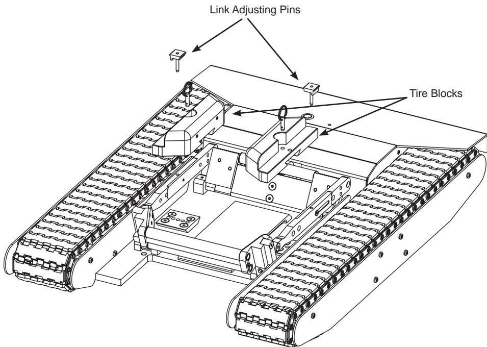
2. Install the Cirrus Tire Blocks with 3 mounting screws on both sides as shown below.
