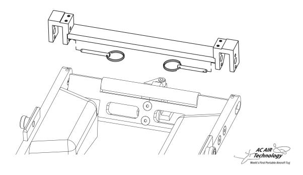
3. Place the roller assembly onto the mount assembly and attach using the four adjustment screws.
