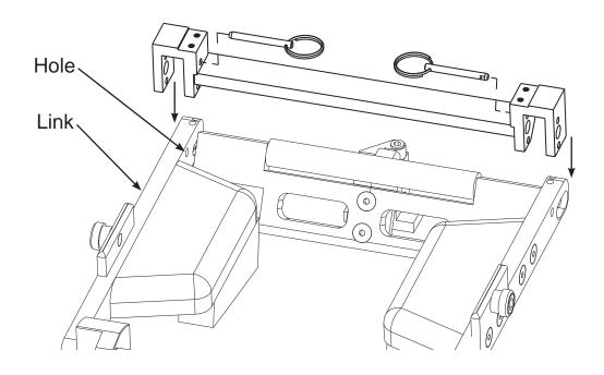
Option 2: If your tug does not have the 1/4" hole on the links then the pins should be inserted into the small lower holes on the mount assembly underneath the links.
